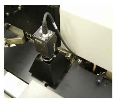
Our Cognex Prealigner Assembly<sup>1</sup> for your Micralign<sup>TM</sup> employs a camera that is able to view the entire wafer, thus eliminating the discrete detectors (A-D). Teamed with our OS2000 Operating System, this allows for:
